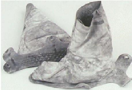
The CPFC are unsupported, impermeable, butyl rubber overshoes that can be stored flat. They are a loose fitting butyl rubber upper vulcanized to a non-slip molded butyl rubber sole with five holes to allow lacing around the foot. They are worn over the combat boot. They have the ability to resist acid, jet fuel, oil and fire. They were manufactured in two sizes, small and large, but are no longer being procured.
