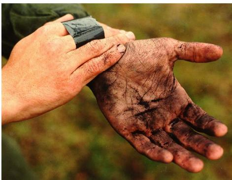
The M291 (shown in use) consists of a wallet-like flexible carrying pouch containing six individually sealed foil packets. Each packet contains a folded non-woven fiber applicator pad with an attached strap handle on one side. The pad contains a reactive and sorptive resin polymer mixture. The kit enables warfighters to remove, neutralize, and destroy chemical and biological warfare agents on contaminated skin. The kit is carried in a pocket of the Battle Dress Overgarment (BDO).
