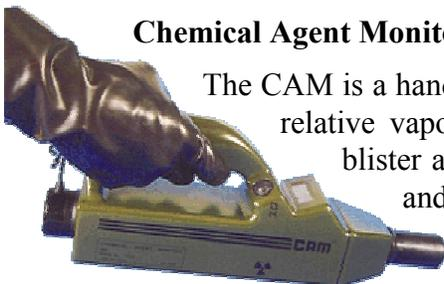
The CAM is a hand held instrument capable of detecting, identifying, and providing relative vapor hazard readouts for G and V type nerve agents and H type blister agents. The CAM uses ion mobility spectrometry (IMS) to detect and identify agents within one minute of agent exposure. A weak radioactive source ionizes air drawn into the system, and the
