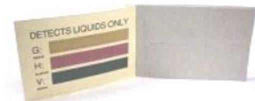
M8 and M9 paper are dye impregnated papers that change color when exposed to liquid chemical agents or aerosols. These papers cannot detect chemical agents in vapor form. M8 paper (*shown*) comes in 4" by 2 1/2" booklets. Each booklet contains 25 sheets of detector paper that are capable
