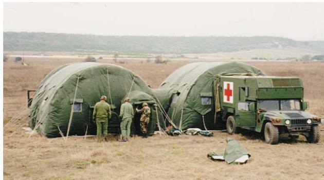
tioned by a hydraulically powered environmental support system, which provides filtered air, heating, air conditioning, and electrical power. The system is presently in limited production.
