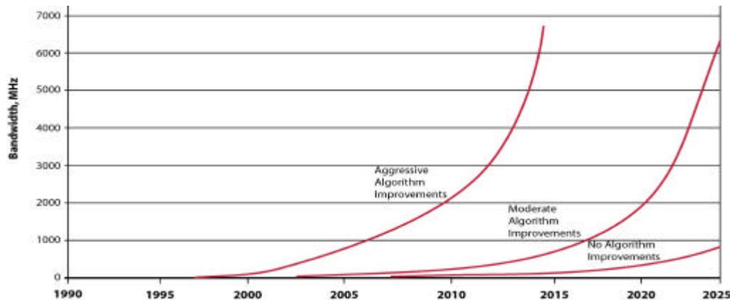
FIGURE 4.2.3-2: FORECAST OF AMOUNT OF BANDWIDTH CONTINUOUSLY PROCESSABLE.
