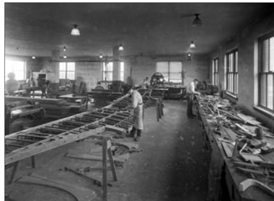
Workmen in the patternmakers' shop at NACA Langley manufacture a wing skeleton for a Thomas-Morse MB-3 airplane for pressure distribution studies in flight, June 1922. The MB-3's wing employed a Royal Air Force 15 airfoil. NASA Image #L-00184 (LaRC)
