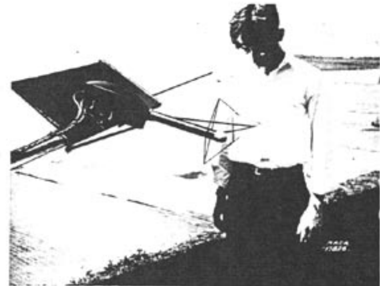
Figure 4.- Wake-survey apparatus installed on the trailing edge of the wing.
