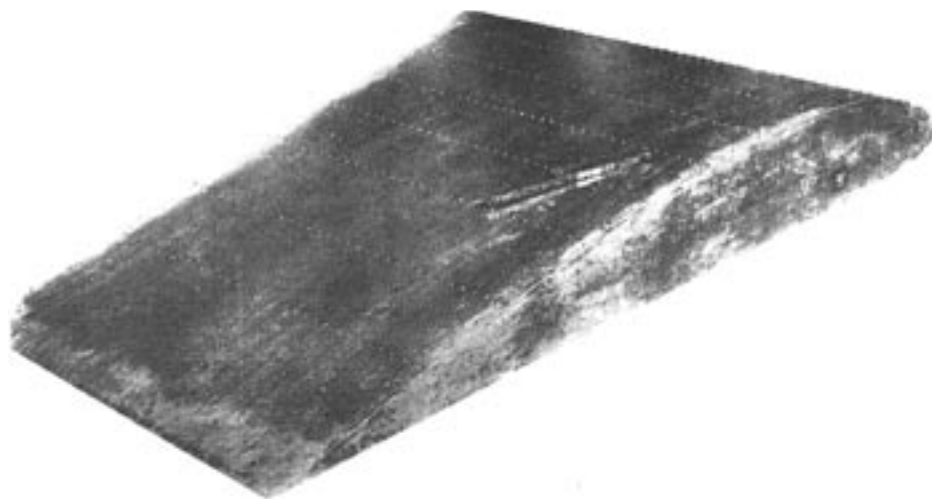
Figure 2.-Nine rows of rivet heads on upper surface of airfoil.
