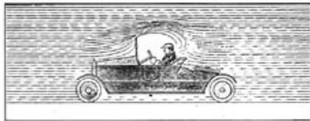
THE AIR FLOW OVER A WINDSHIELD VISUALIZED
