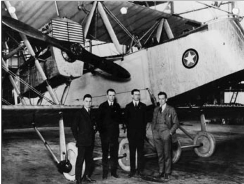
Aircraft such as the biplane, strut-and-wire braced Martin MB-1 Bomber represented the state of the art in aerodynamic design circa 1917. The designers of the aircraft, Laurence D. Bell (left), Glenn A. Martin (second from right), Donald W. Douglas (right), and James Kindelberger (not pictured), would use the advances of the design revolution to create vastly different aircraft. (Martin test pilot, Thomas E. Springer, is second from left.) (SI Negative No. 43067)
