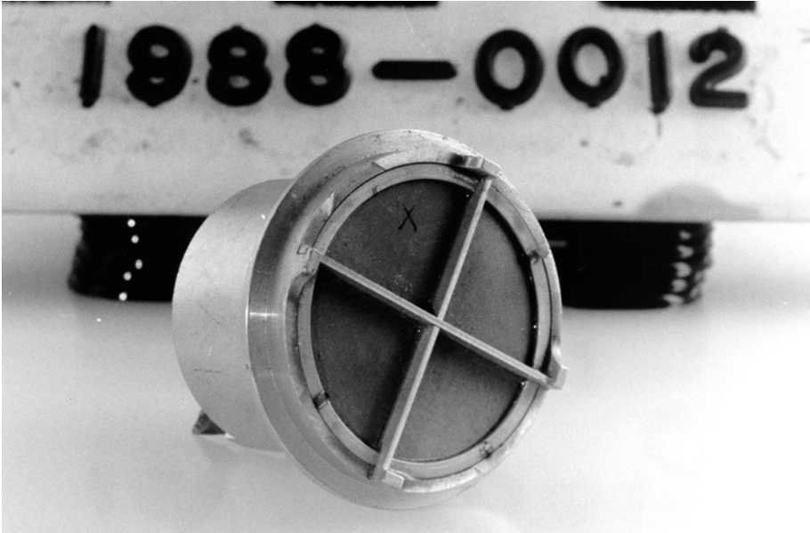
Typical x-ray ionization chamber designed, built, and used by the Naval Research Laboratory team on sounding rocket flights in the 1950s and early satellite systems. ( File no. A1988-0012000, NASM Curatorial Files )
