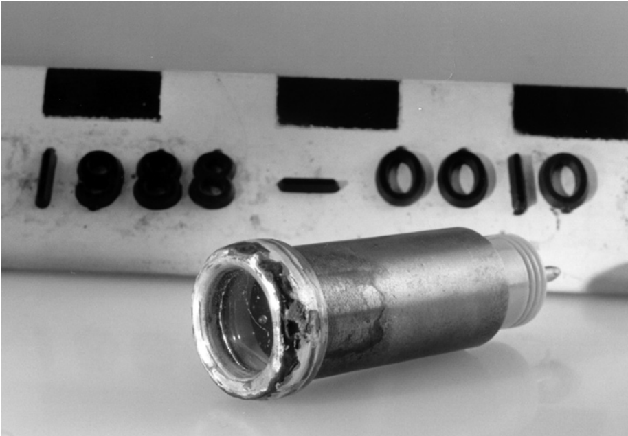
Early halogen counter with an entrance window of mica, capable of sensing ionizing ultraviolet radiation. Note the suspended anode just behind the mica window. This is a tube similar to the one Kreplin tapped during his video-history interviews. ( File no. A1988-0010000, author digital file, NASM Curatorial Files )
