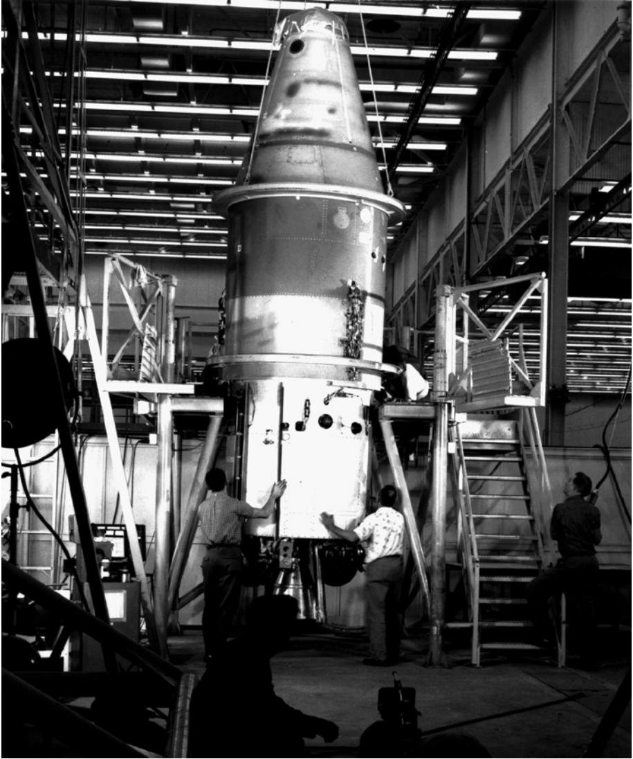
An Agena A spacecraft for an early MIDAS launch undergoes a weight test in 1960 at Lockheed's plant in Sunnyvale, California, before shipment to Cape Canaveral for launch. ( Official USAF photo. Air Force Space Command, Office of History )
