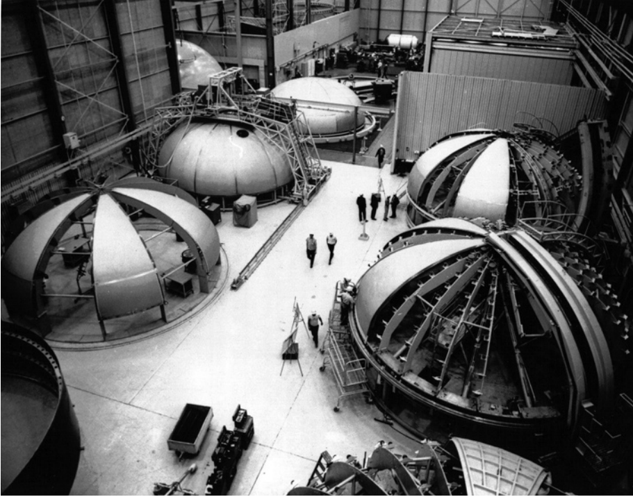
Gores being welded to bulkheads for the S-II stage of the Saturn V. (Source: Roger Bilstein, Stages to Saturn [Washington, DC: NASA SP-4206, 1980; reprint, Gainesville: University Press of Florida, 2003], p. 221)
