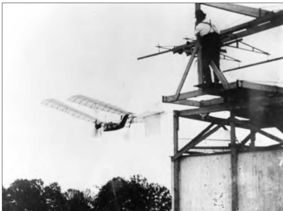
The successful launch of Langley's Aerodrome No. 5 from atop a houseboat in the Potomac River, on 6 May 1896. SI Negative No. A-18870
