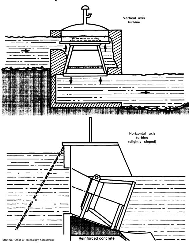
Figure 36.- Vertical and Horizontal Axis Turbines
