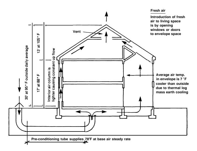
Figure 12.—Thermal Envelope House, Ventilation and Cooling Cycle
