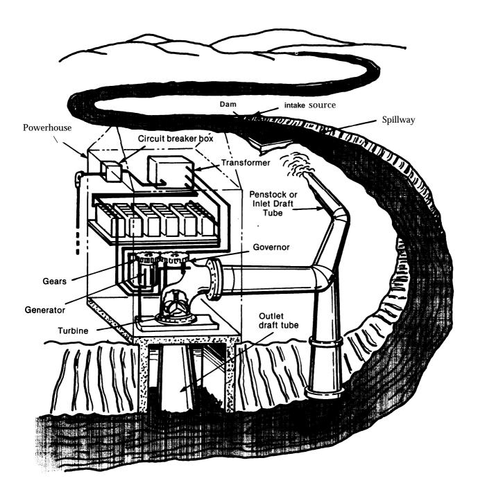
Figure 34.—Low Head Hydroelectric installation
