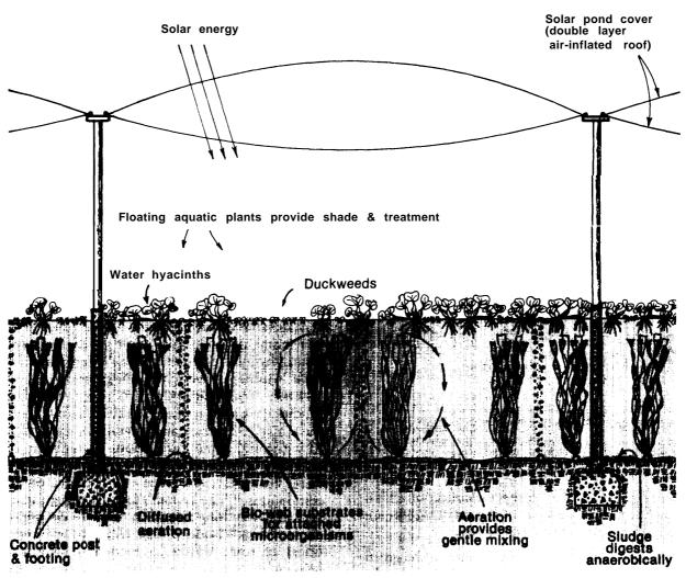
Figure 29.—Section View, Solar AquaCell System
