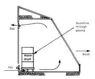
Thermal Flow Diagram of the Hinesberg Greenhouse
