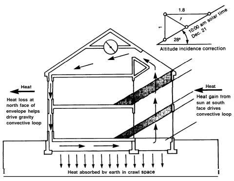
Figure 10.—Thermal Envelope House, Heat-Gain Cycle
