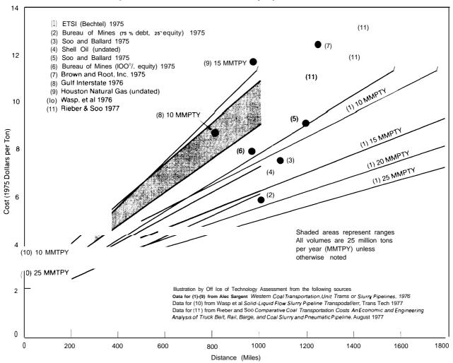
Figure 16- Results of Previous Coal Slurry Pipeline Cost Studies
