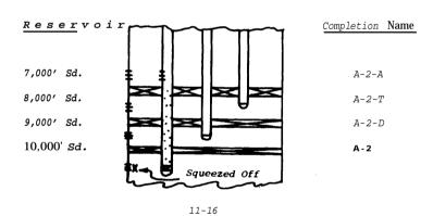
Example No. If 5the A-2 completion in Example No. 4 had. been completed from the 10,000' sand to the 9,000' (where the A-2-D is currently completed), the pletion would still be named A-2-D as both tub strings would be considered one completion fo poses of this Order.
