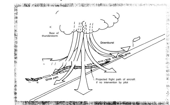
The downburst spreads out as it nears the ground. The aircraft, instead of following a straight path to the runway, encounters first an abrupt increase in headwind which lifts the nose, and then a sudden strong tailwind, which forces the nose down. If the pilot cannot compensate for these wind changes at low altitude, the aircraft may crash.
