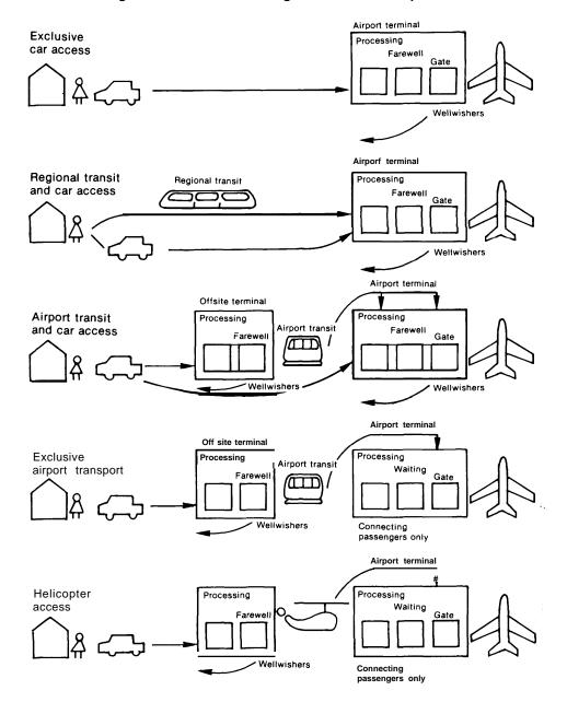
Figure 15.—Off-Site Passenger Terminal Concepts
