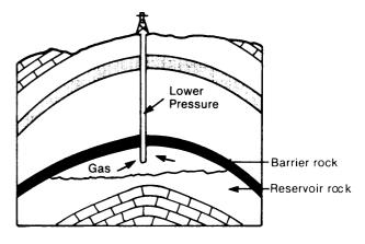
Gas and water drive mechanism
