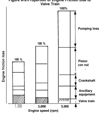
Figure A-2-Proportion of Engine Friction Due to
