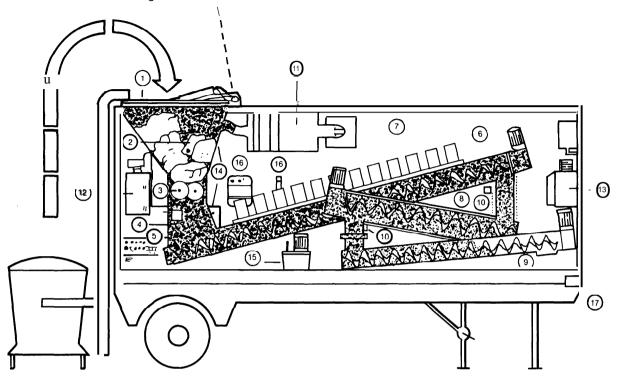
Figure 6-Mobile Microwave Medical Waste Disinfection Unit
