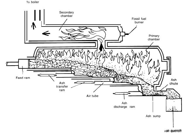
Figure 8-Controlled Air Incinerator
