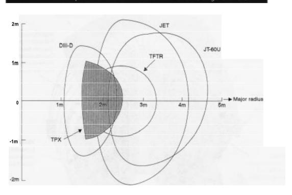
FIGURE 3-2: Comparison of Plasma Cross-Sections of Selected Large Tokamaks
