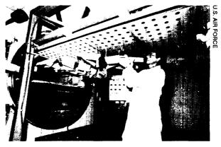
U.S. Air Force ion vapor deposition R&D. Although most DOD environmental R&D is for remedial clean-up of contaminated sites, some work is dedicated to developing advanced manufacturing processes that lessen environmental impacts.
