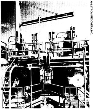
Oxygen reactors, part of an oxygen delignification system in a pulp mill.
