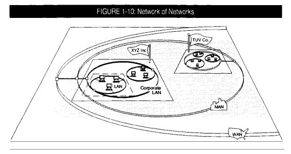
This figure Illustrates how the data communications portion of the information superhighways composed of a complex network of interconnected networks A firms internal computer network typically consists of several smaller, linked local area networks (LANs), which in turn are Interconnected to increasingly wider networks, MANs and WANs
