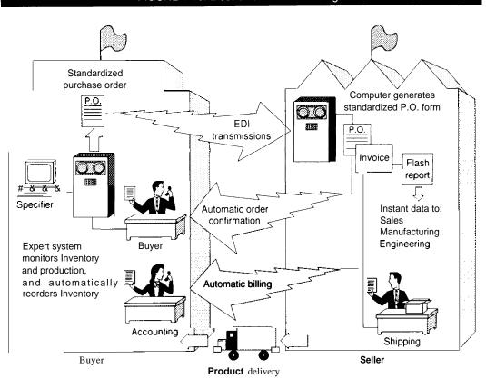
FIGURE 1-13: Electronic Data Interchange
