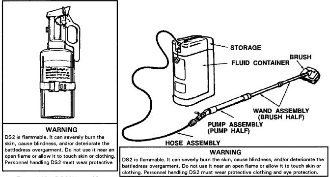
Figure 1-28. ABC-M11 portable decontaminating apparatus.
