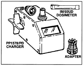
Figure 1-23. IM93/UD dosimeter and PP1578A/PD radiac-detector charger.
