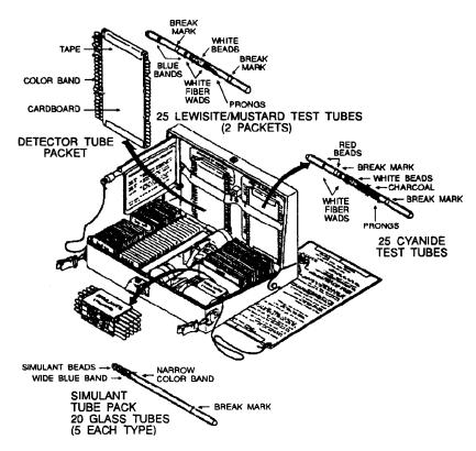
Figure 1-24. M272 water testing kit.
