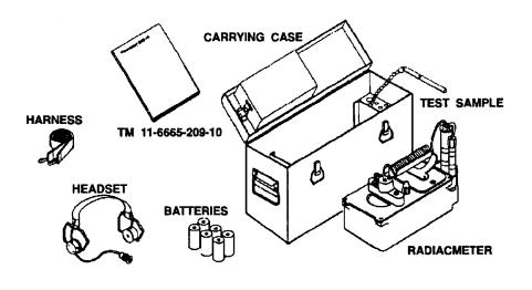
Figure 1-27. AN/PDR27 radiac set and components.
