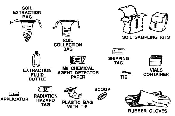
Figure 1-22. M34 soil sampling kit.
