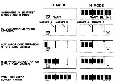
Figure 1-21. Description of CAM displays.
