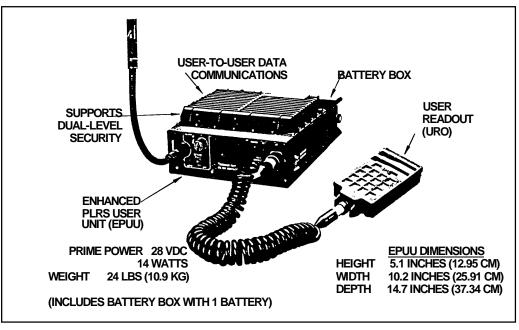
Figure 6-3. Enhanced Position Location Reporting System (EPLRS)
