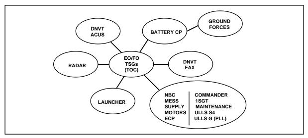
Figure 4-11. Battery Wire/Telephone Net
