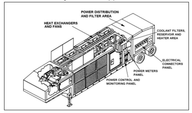
Figure 4-4. Cooling Equipment Unit
