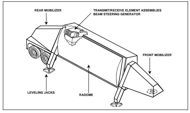
Figure 4-2. THAAD Antenna Equipment Unit
