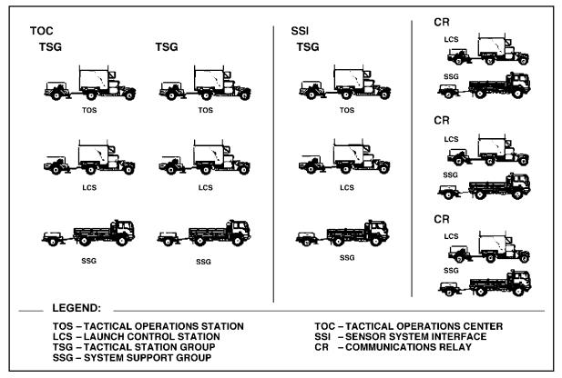
Figure 4-6. Battery BM/C3I Configuration
