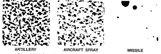
Figure 1-2. Moderate liquid contamination on M9 paper (1 gram/square meter).
