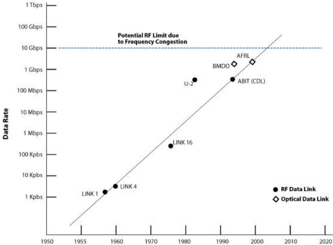
FIGURE 4.3-2: AIRBORNE DATA LINK DATA RATE TRENDS.
