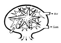
6. Residual heat from the initial combustion ignites the second and subsequent air/gas mixtures without the need for the spark plug or blower...at a ratein excess of 25 cycles per second.
