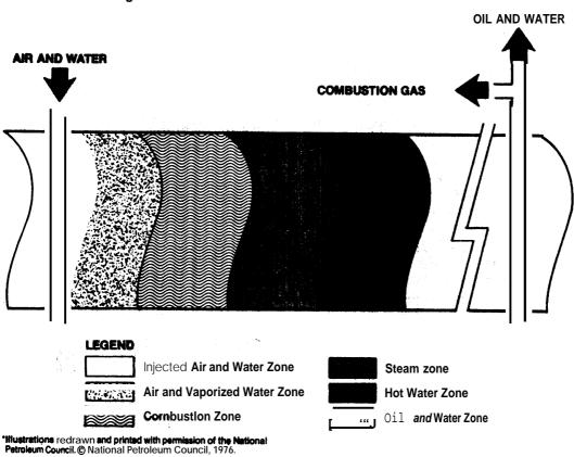
Figure 10. In-Situ Combustion Process-Wet Combustion\*
