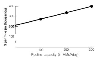
Pipeline Investment Costs *per* Mcf.—The cost -capacity graph was translated into a cost per Mcf (per 100 miles) graph by dividing costs by capacity, as follows:
