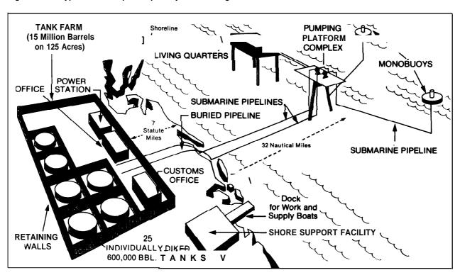
Figure IV-42. Hypothetical deepwater port layout including onshore facilities
