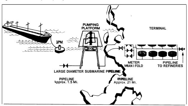
Figure IV-37. LOOP deepwater port layout
