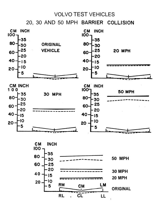
FIGURE 5: HOOD AND BUMPER DEFORMATION FROM STAGED FRONTAL BARRIER COLLISIONS.
