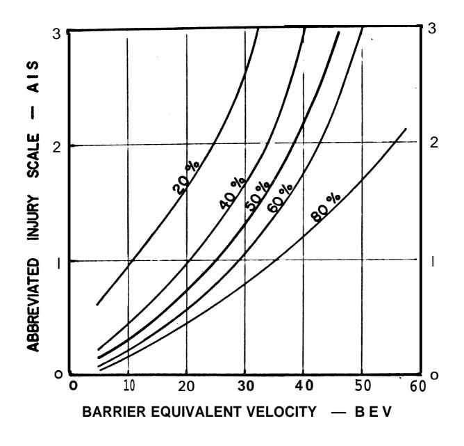
FIGURE 9 : INJURY AS A FUNCTION OF BARRIER EQUIVALENT VELOCITY FOR CUMULATIVE PER CENT OF INJURY
