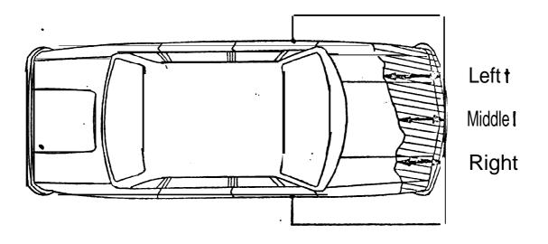
FIGURE 4 : DIAGRAM SHOWING MEASUREMENTS TAKEN WITH FRONT END DEFORMATION FIXTURE.
