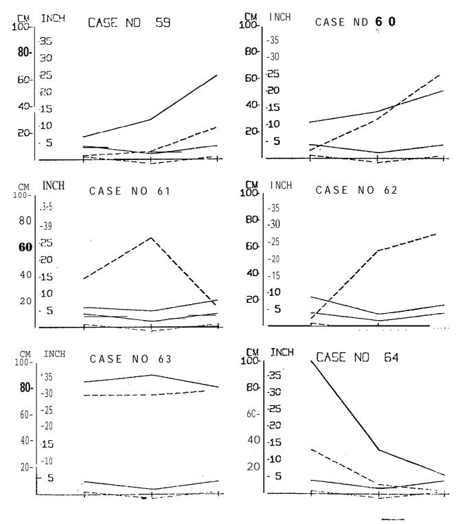
'FIGURE 6 : " DEFORMATION DATA FROM EIGHT OF THE ACCIDENT CASES .
