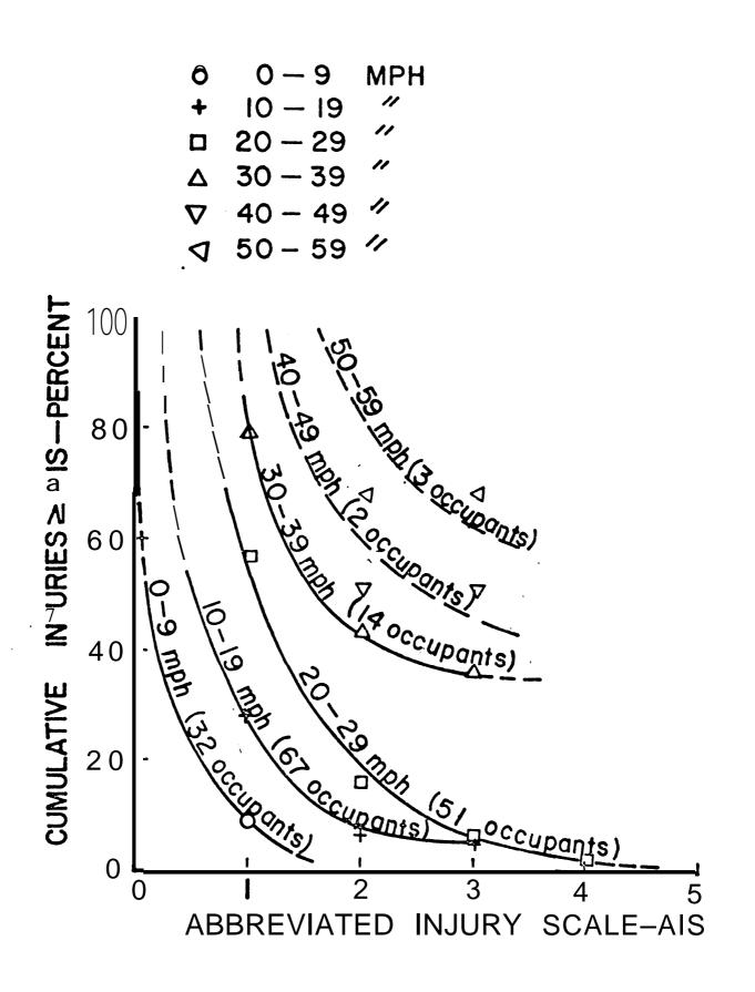
FIGURE 8: PERCENT OF CUMULATIVE INJURIES, EQUAL TO OR GREATER THAN, A GIVEN AIS LEVEL FOR 10 MPH INCREMENTS .
