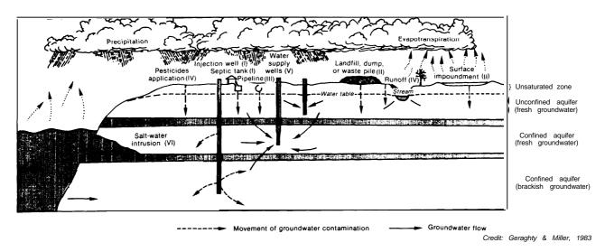
Pathways of groundwater contamination vary depending on the source. Examples of sources are shown here for each of OTA'S six source categories (I-VI) (see the section on Types of Sources and Associated Substances, below).
