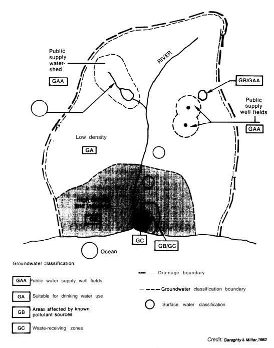
Groundwater classification schemes are used to facilitate decisions about groundwater quality protection in some States. The example shown illustrates the groundwater classification system applied by the State of Connecticut.
