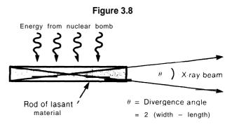
Figure 3.8 In an x-ray laser, a rod of lasant material is pumped to upper energy states by a nuclear bomb. Those cascades of downward transitions that travel lengthwise build up more energy than sideways-going cascades. As a result, most of the energy emerges from the ends of the rod into a cone with divergence angle equal to twice the rod width divided by its length. Source: Author
