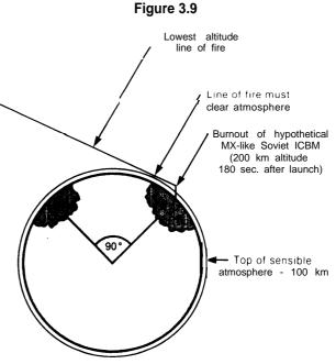
Figure 3.9 X-ray lasers launched from the United States on warning of Soviet ICBM launch would have to climb at least as high as the line of fire shown in the figure within three minutes to intercept an MX-like Soviet ICBM. Such a huge fast-acceleration defensive booster would be many times larger than the Saturn V that took astronauts to the moon. Source: Author
