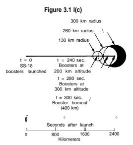
(c) The High Frontier Global Ballistic Missile Defense (GBMD) concept, with intercept vehicles capable of only 1 km/see velocity relative to the satellite. Intercept of SS-18. In the actual High Frontier proposal, the satellites are in 600 km orbits, giving them even less coverage than shown here.
