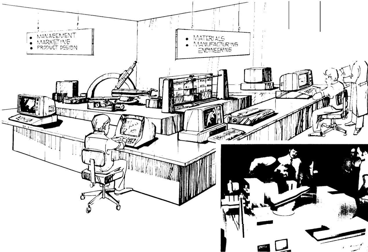
This is a scale model (inset) of the group technology cell that will be a part of BYU's "CAM Mini-Lab." The model was built in the University's Research Laboratory (see caption below)
