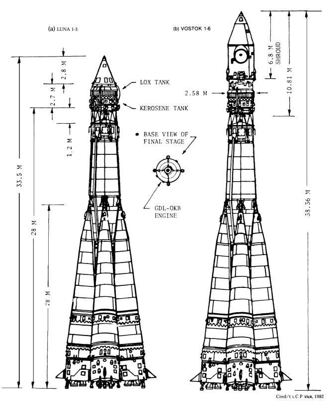
Luna 1-3 (a); Vostok 1-6 (b) —standard launch vehicle with the first type of added upper stage A-1 (a) as used to launch the first three Luna spacecraft; (b) as used to launch the six Vostok manned spacecraft
