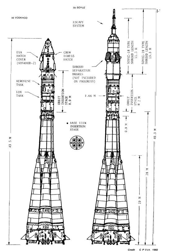
Voskhod-2 (a); Soyuz T (b) —standard launch vehicle with the improved upper stage A-2 (a) as Jsed to launch the two Voskhod manned spacecraft; (b) as used to launch the Soyuz T manned spacecraft
