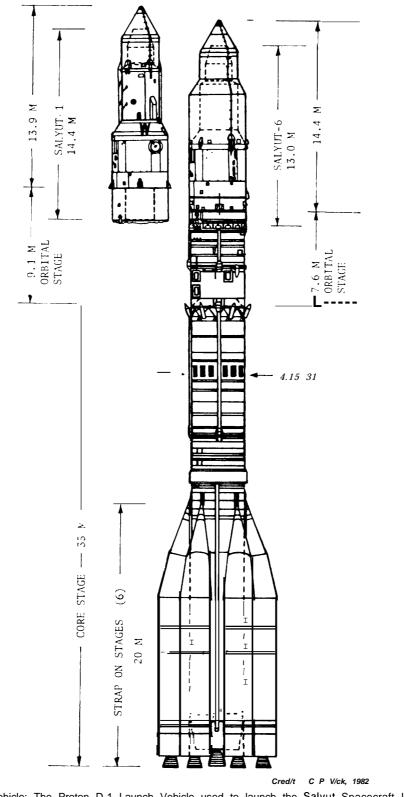
Salyut launch vehicle: The Proton D-1 Launch Vehicle used to launch the Salyut Spacecraft Laboratory. It is a three-stage launch vehicle
