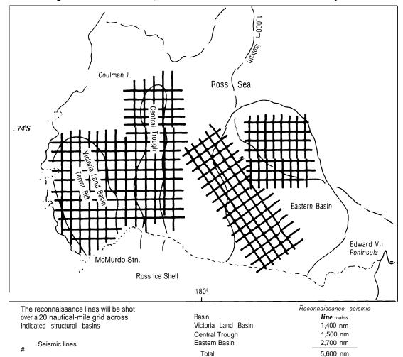
Figure A-I—The Ross Sea, Antarctica: Reconnaissance Seismic Survey Lines
