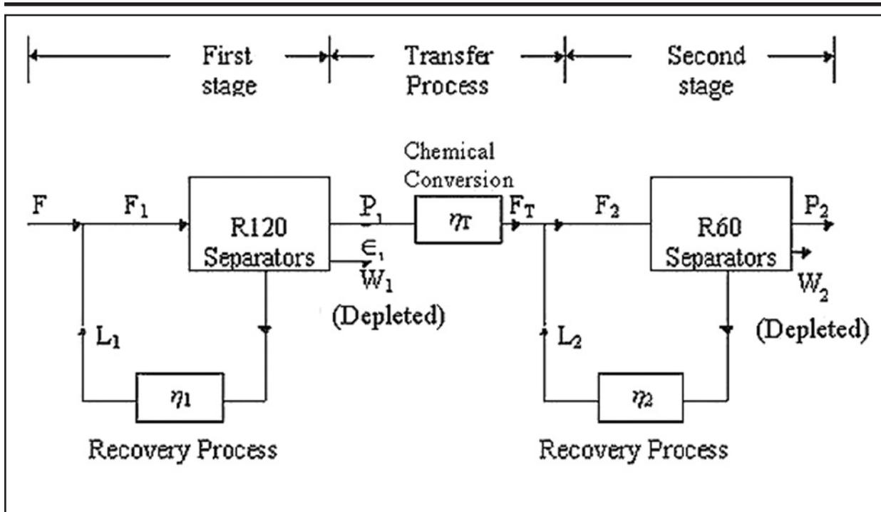
Figure 21. Flow diagram of the Iraqi EMIS process.
