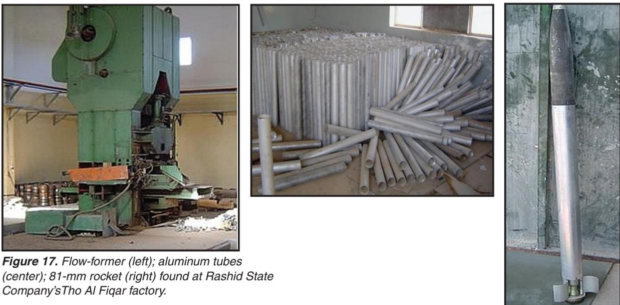
**Figure 17.** Flow-former (left); aluminum tubes (center); 81-mm rocket (right) found at Rashid State Company's Tho Al Fiqar factory.
