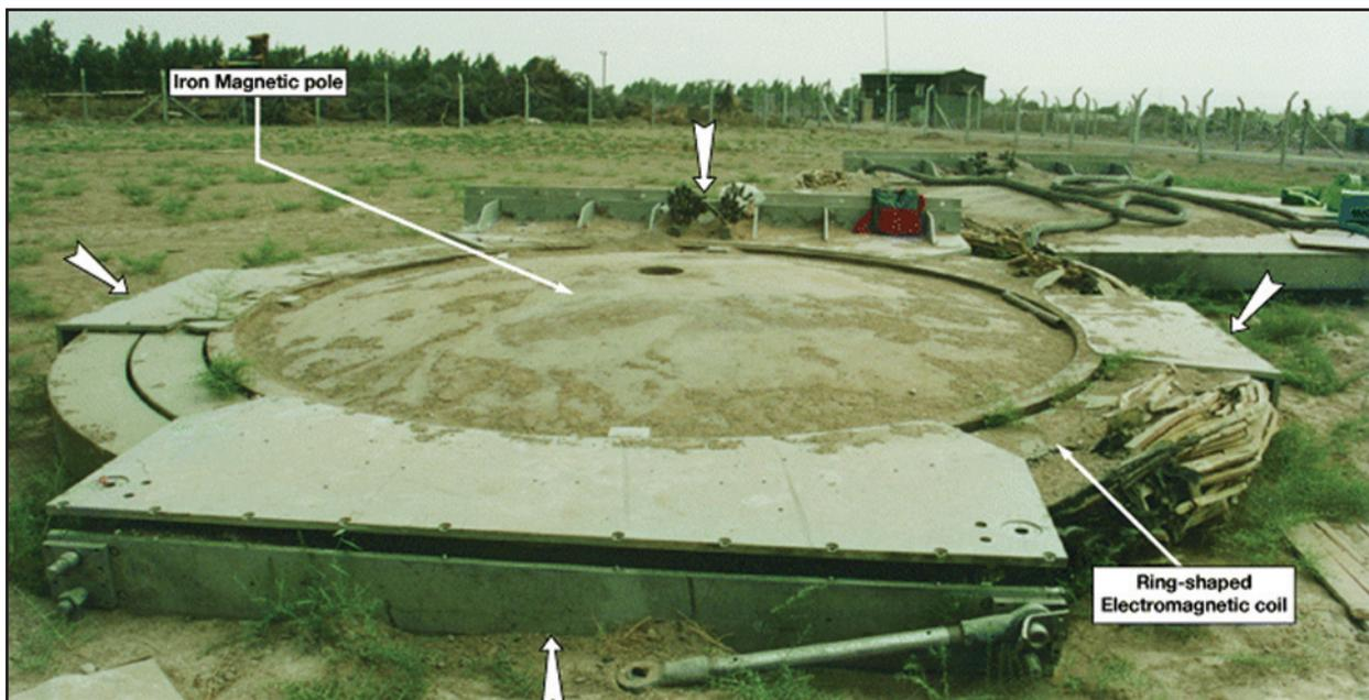
Figure 19. Photograph of Iraqi EMIS electromagnet.
