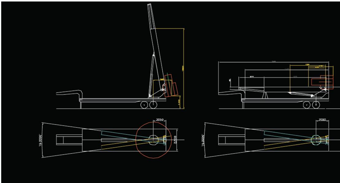
**Figure 20.** Designs for long-range solid-propellant missile launcher.
