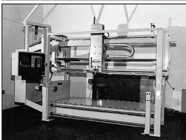
Figure 11. Example of horizontal filament winding machine.
