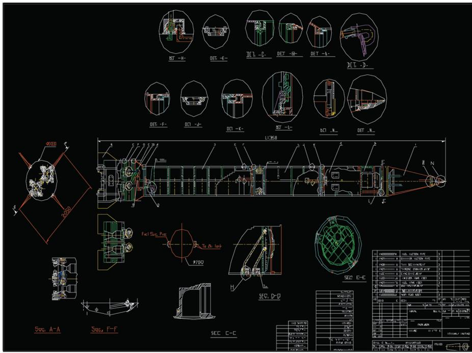
Figure 18. Design drawings for two-and five-engine cluster missile.
