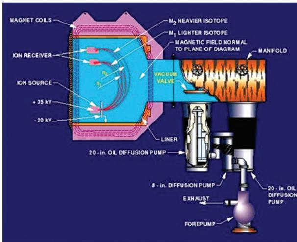
Figure 18. Example of EMIS separator and vacuum system.
