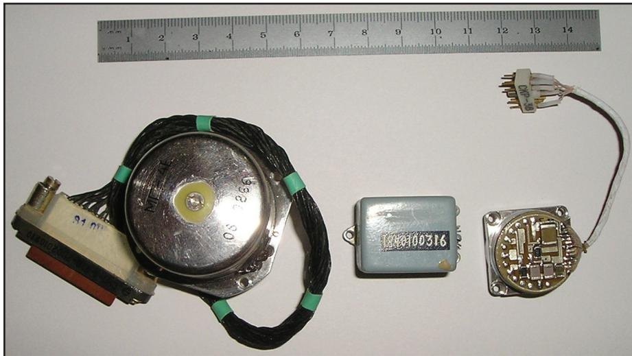
Figure 28. MG-4 gyroscope,
