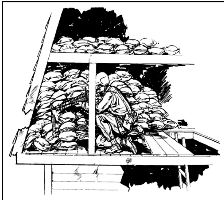
Figure 3-60. Firing platform built under roof.
