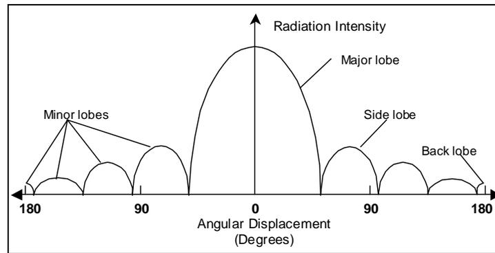
**Figure 1: Example of an Antenna Pattern <sup>23</sup>**
