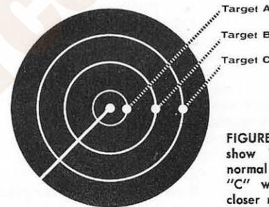
FIGURE 8B: The radarscope will show Targets "A" and "B" at normal range, but distant Target "C" will appear to be at much closer range than it actually is.
